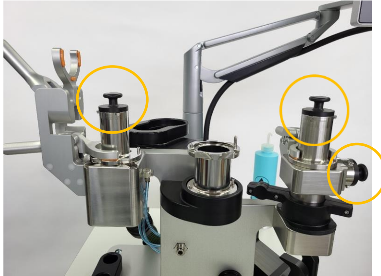
Closed and protected particle suction extraction system, cyclone unit, and filter unit
