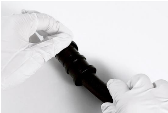
Covering hose ends with plugs
