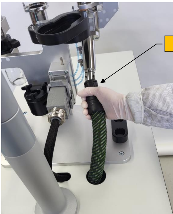
Connecting Festool hose to suction unit
