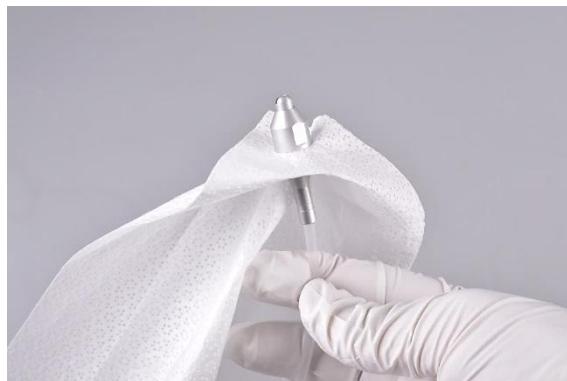
Cleaning wire with attached alcohol-soaked cleaning cloth
