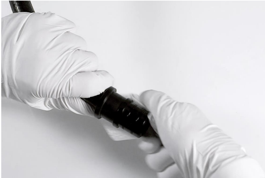
Cleaning the connectors on the end of the hose
