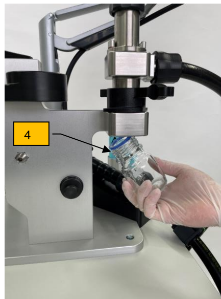
Replacing the particle collection jar
