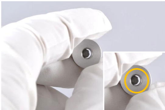
Blocked cone thread
