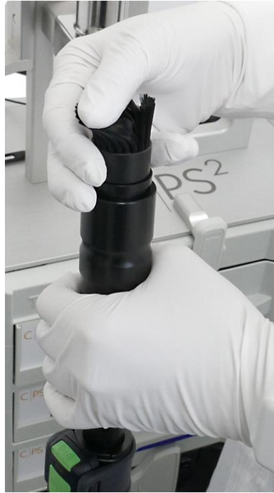
Pre-cleaning the brush suction nozzle mechanically
