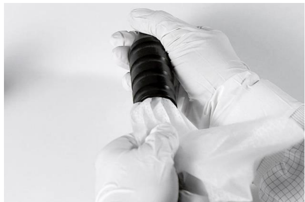
Cleaning the suction nozzle
