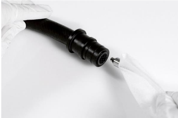
Inserting the alcohol-soaked cleaning cloth
