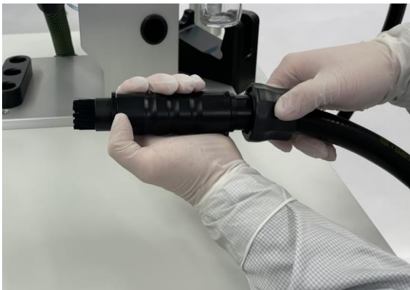
Attaching the suction nozzle
