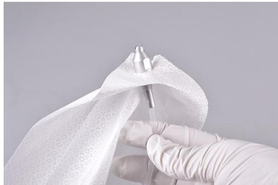
Cleaning wire with attached alcohol-soaked cleaning cloth
