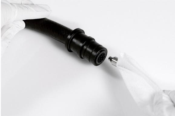
Inserting the alcohol-soaked cleaning cloth
