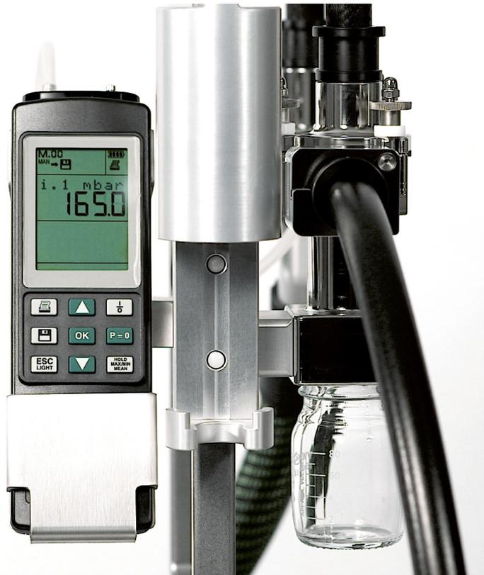
The differential pressure measuring device
