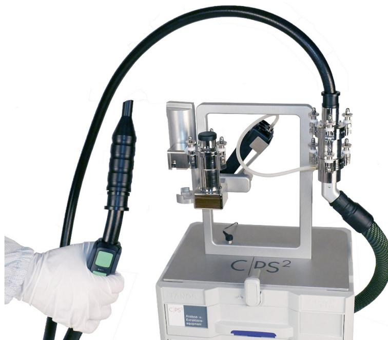
Determining the blank value, suction from the atmosphere
