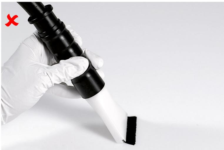
Applying the flat nozzle incorrectly
