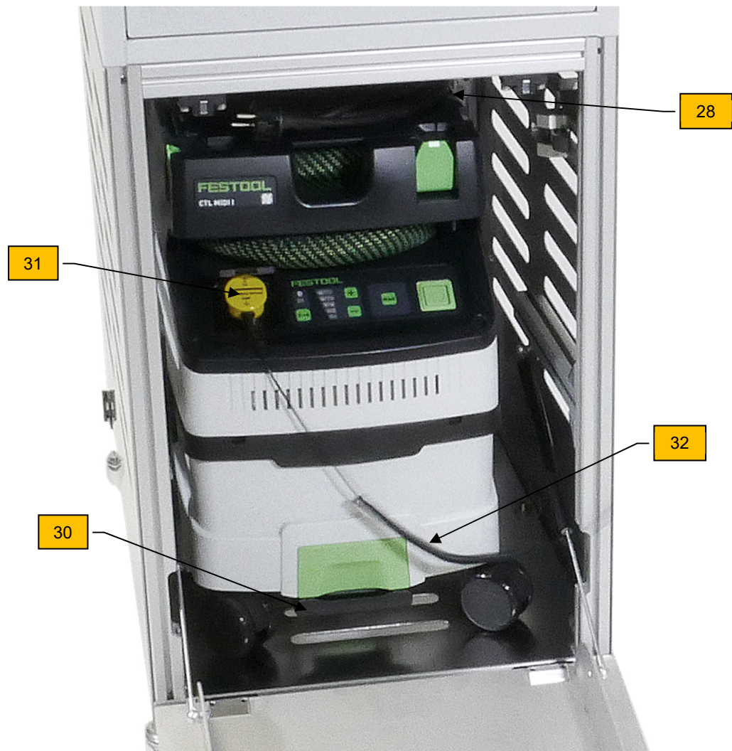
Connecting the grounding cable
