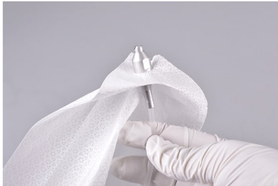
Cleaning wire with attached alcohol-soaked cleaning cloth
