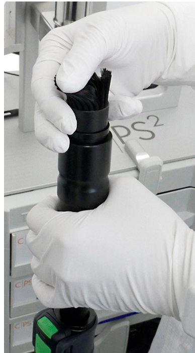
Pre-cleaning the brush suction nozzle mechanically
