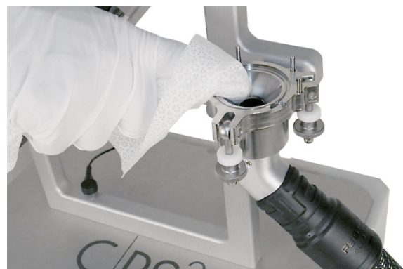
Cleaning cyclone unit and filter unit on the inside and outside
