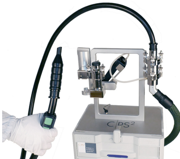
Determining the blank value, suction from the atmosphere
