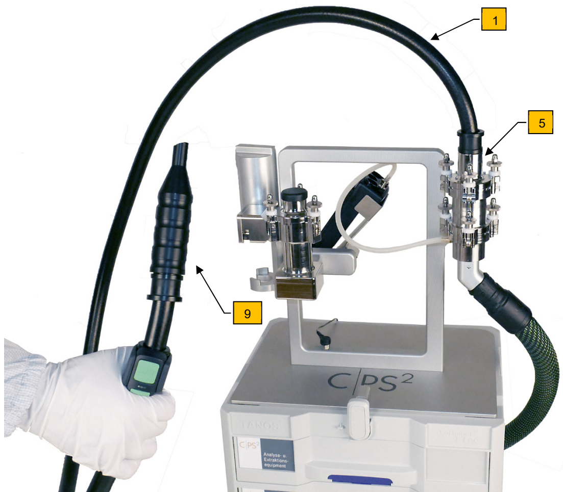
Attaching the suction hose and suction nozzle
