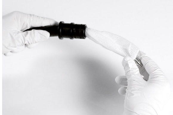
Alcohol-soaked cleaning cloth pushed through
