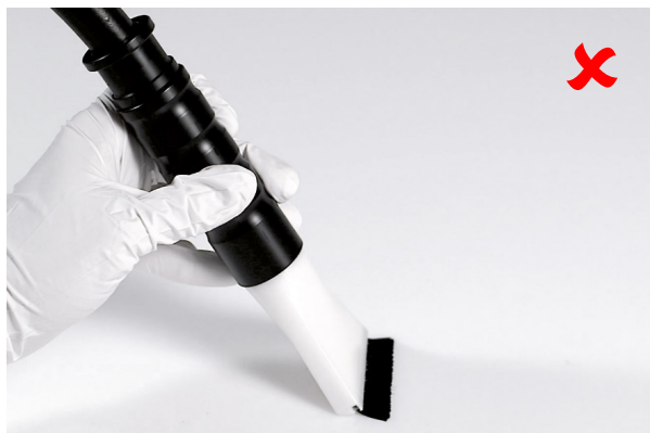
Applying the flat nozzle incorrectly
