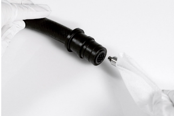
Inserting the alcohol-soaked cleaning cloth
