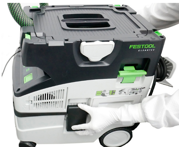
Replacing the mobile dust extractor filter
