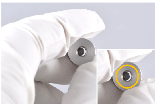
Blocked cone thread
