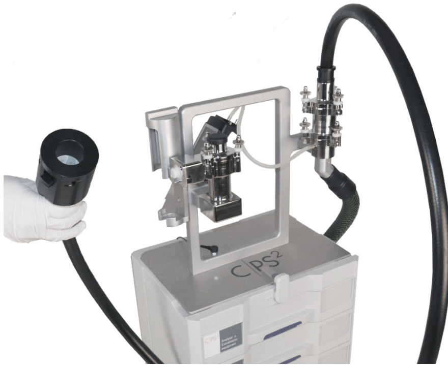
Determining the blank value, suction with prefilter
