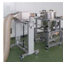
Construction of an air extraction test bench for air-conducting components in accordance with VDA 19.1 as the world's first laboratory service provider
